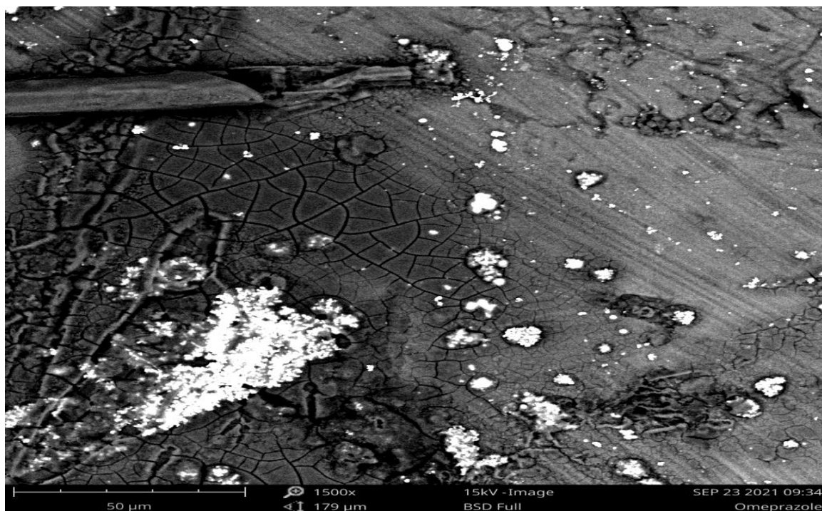
Figure 3: SEM for Omeprazole-silver nanoparticles
